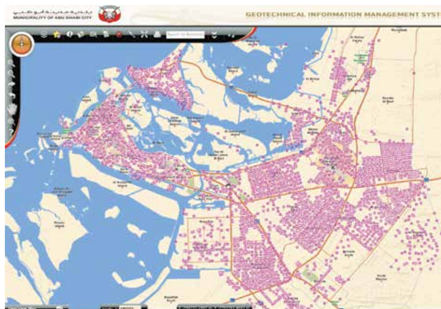
Figure 3. The Geotechnical Information Management System (GIMS) provides easy access to data for all boreholes around Abu Dhabi City.
