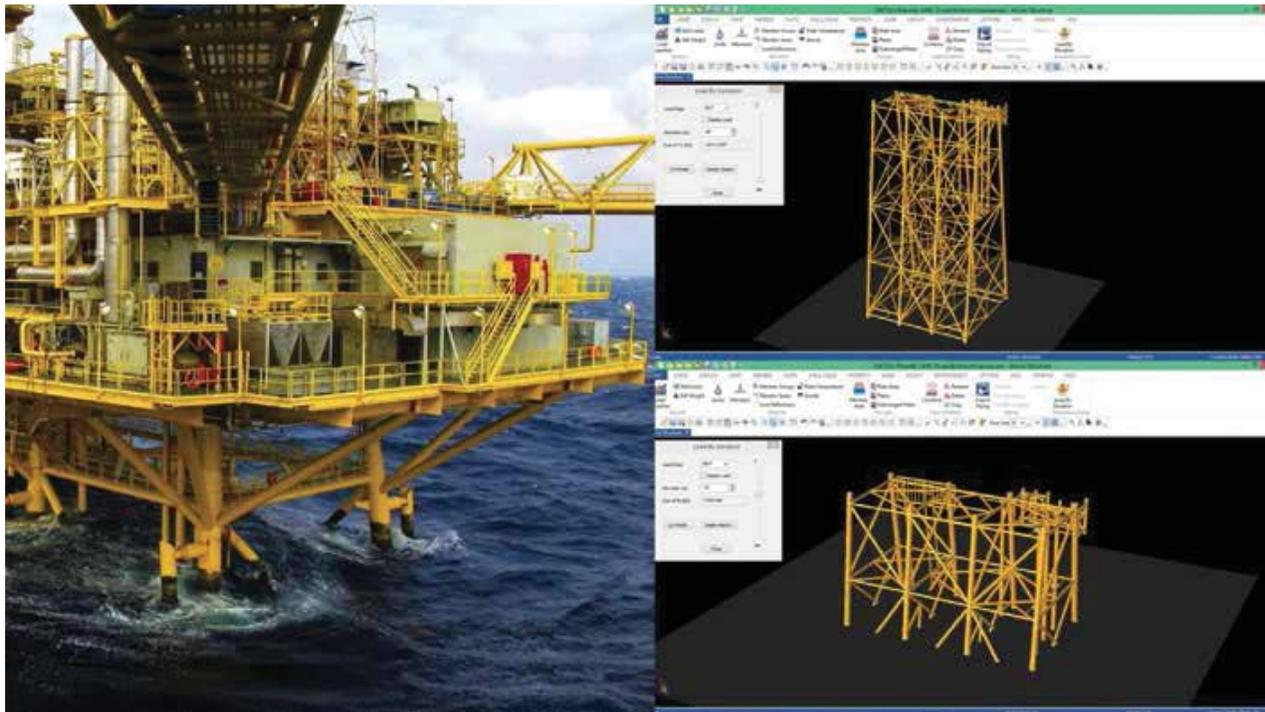
The interoperability between AutoPIPE and SACS enables complete piping designs for offshore structures in hours, not weeks.
