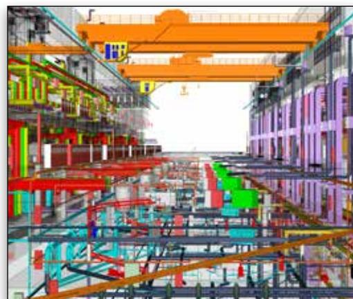
PowerChina Huadong Engineering Corporation used Bentley Raceway and Cable Management for layout, routing, and material estimating.
