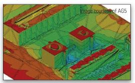
Energy calculations and simulations, in this case a solar exposure study, was done over a whole year which provided clues on how to the sun shading could look like based on how many hours of sun the facade got
