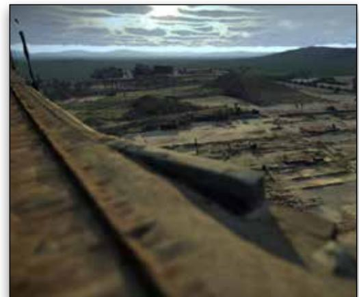
*CEDARVILLE captured more than 750 aerial photos via a drone in a matter of 20 minutes, and using ContextCapture, incorporated base imagery to build a precise reality model.*
