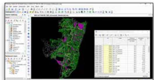
The WaterGEMS hydraulic model replicated distribution schemes in varying zones and assessed various what-if simulations
