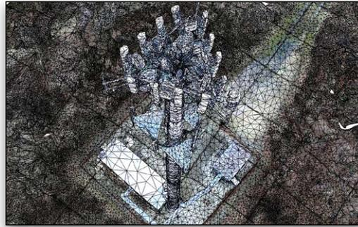
*A 3D reality mesh generated from UAV photogrammetry and LiDAR scans.*
