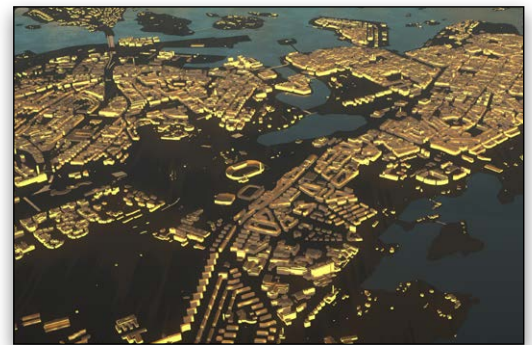
ContextCapture enabled Helsinki to produce the final detailed 3D reality model with an overall accuracy of up to 20 centimeters.
