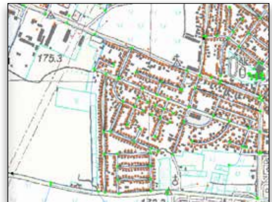
The WaterCAD model was integrated with GIS and other data sources to ensure accurate model data and a reflection of reality.
