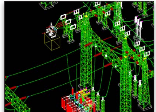
iSAT integrated 2D electrical design, 3D physical layout, and structural design using Bentley Substation and STAAD.Pro.
