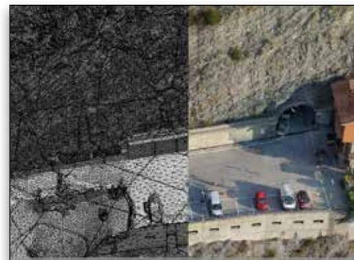
*ContextCapture's SfM imaging technique aligned 2D photographic images of the dam and ancillary buildings in a 3D geo-referenced space to create 3D models of the structures.*
