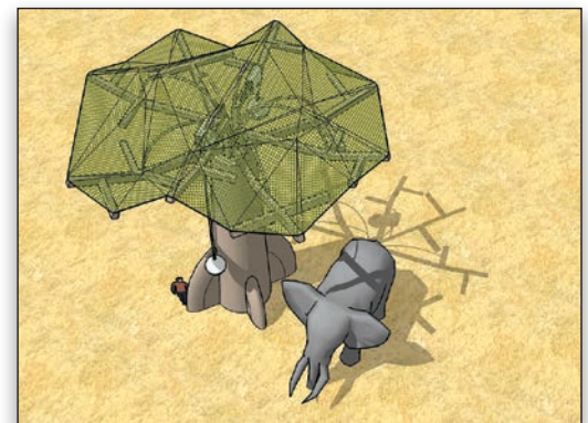
This is a top view rendering of the shade structure. The hoists that raise and lower the enrichment devices can be seen in this view.
