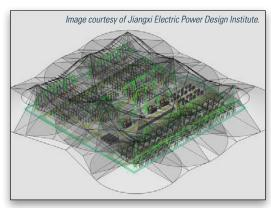
The 3D substation model enabled lightning protection modeling and visualization.
