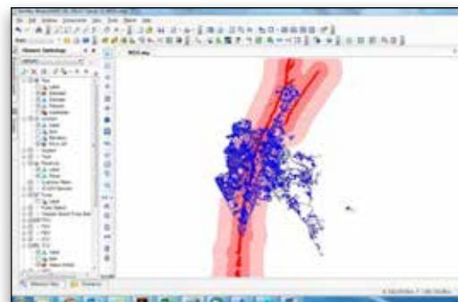
*WaterGEMS was used to create a model that overlaid pressure and flow profiles on a GIS-based map, which helped the project team find the areas that have reliable water supplies.*
