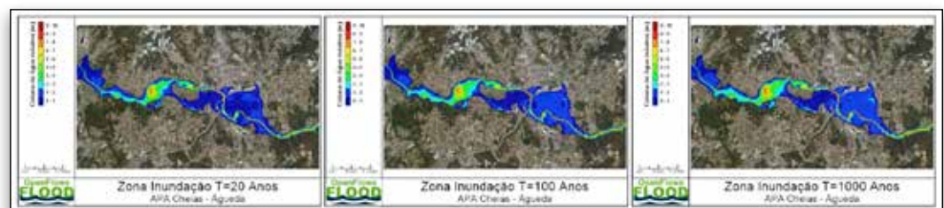
The image shows the maximum water depth for three different return periods.
