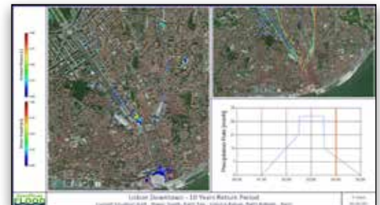
Flood simulation in downtown Lisbon. The image shows ponded water on the surface (on the left), capacity of the stormwater system (upper right), and the design storm (lower right).
