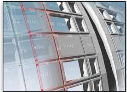
Depiction of the innovative bent-glass cladding system.
