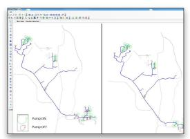
Modeling current and future scenarios in WaterGEMS optimized pipeline sizes, pressure ratings, bore pump run time, and other factors to meet changing operational requirements at minimal cost.
