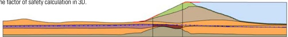
Figure 1 - Cross section of lithology, tailings dam, and tailings.
