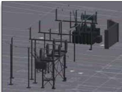
*Bentley Substation allows PG&E to combine legacy vector and raster drawings with 3D equipment models to intelligently design brownfield projects.*
