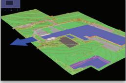
SITEOPS allowed Manhard to provide a grading design that minimized the volume of earth moved, significantly reducing the time associated with preparing the site for building erection.
