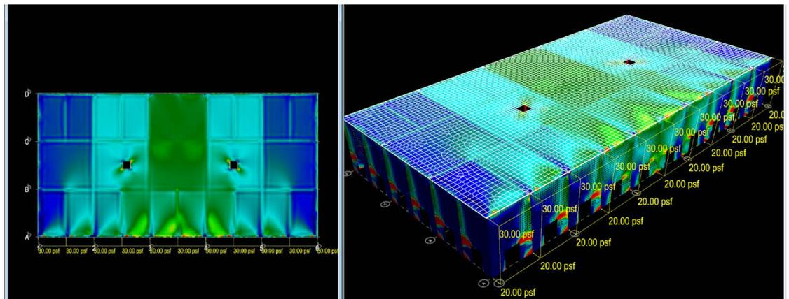
**Image 4:** The internal force contour plot depicts the transfer of the wind load acting on the exterior wall from the “south” side of the building into the semirigid diaphragm.
