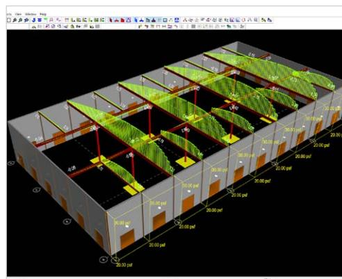
**Image 5:** The RAM Frame view demonstrates the axial forces developed in the cross ties and chords for the load considered.
