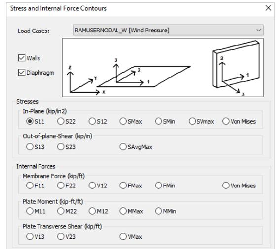
**Image 3:** RAM Frame provides a dialog to display stress and internal force contours.
