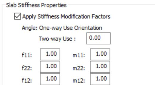
**Image 2:** Stiffness modification factors can be specified in RAM Modeler.
