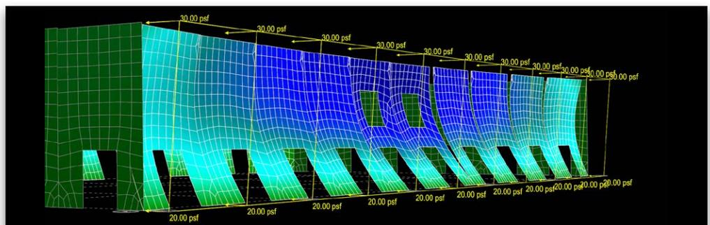
**Image 1:** RAM Frame depicts the deflected shape of the structure responding to a windward lateral wind pressure.
