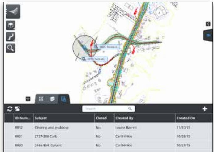
*OpenRoads Navigator makes it easy to work with 2D or 3D designs while in the field allowing you to access all project information associated with the project.*
