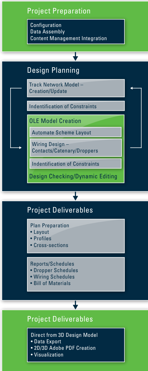
Overhead Line System – Design Process.
