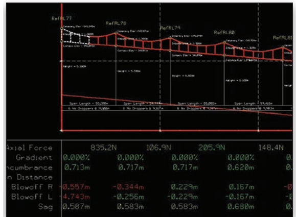
View, analyze and adjust height, stagger and wire gradient via an interactive, graphic interface.
