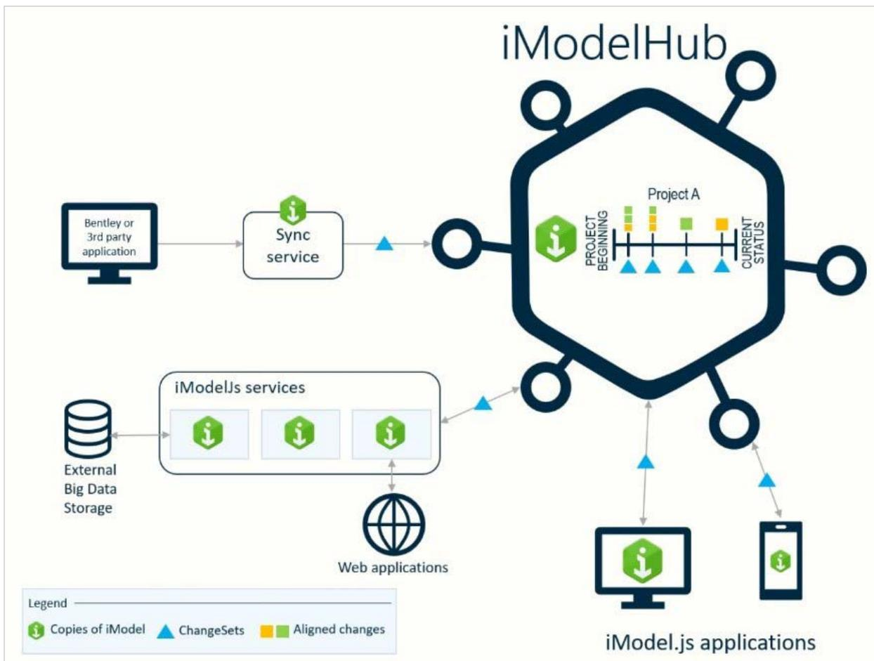
**Figure 1. iModelHub is the control center for iModels, responsible for coordinating concurrent access to iModels as well as changes made to them in a form of ChangeSets.**
