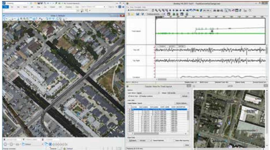
Figure 6: Synchronization of CAD (left), Linear Data (Top Right), EAM (Bottom Middle), and Maps (Bottom Right)
