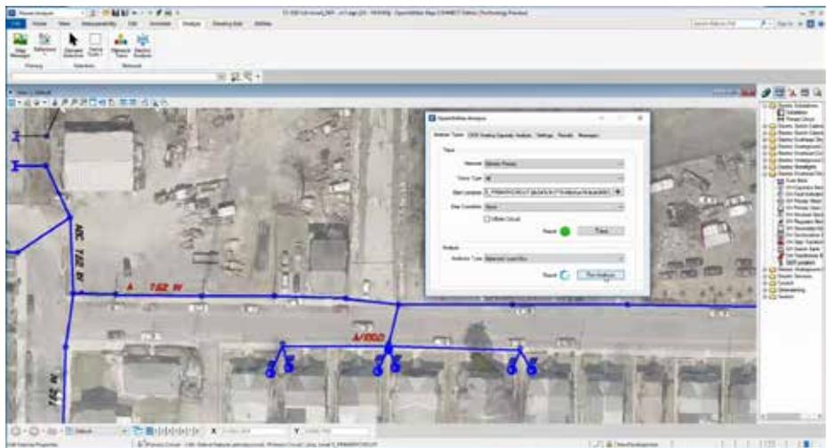
Figure 6: Network load analysis embedded in a GIS-based network design workflow.
