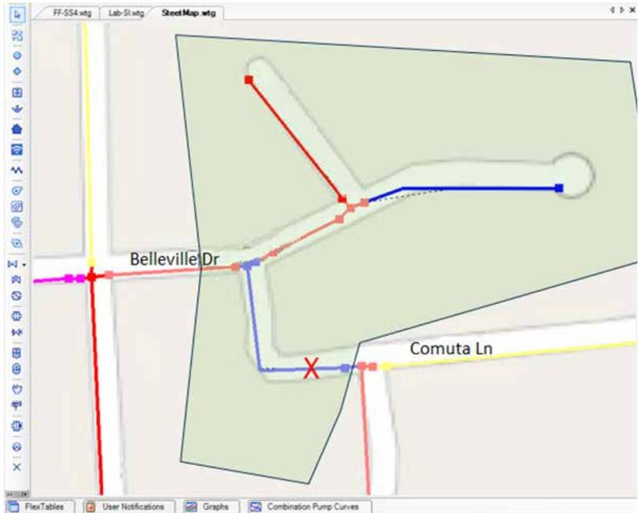
Figure 4: In complex networks, a shutdown map similar to this one can be provided to operators. Because of valving at the intersection of Belleville Dr. and Comuta Ln., all of the customers in the green box would be cut off from water during a shutdown, not just those served directly by the pipe with the "X."
