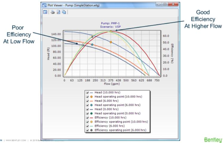
Figure 5: Users can view pump operating points to ensure that they are working at optimal efficiency.
