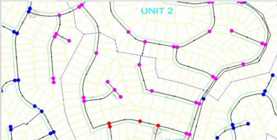
Figure 7: A color-coded map in WaterGEMS, showing customers with excessive pressure along the pressure zone boundary. Magenta nodes are in the higher zone, blue ones in the lower zone, while red ones are in the higher zone but have high pressures and may be better off being moved to the lower zone by adjusting valves.
