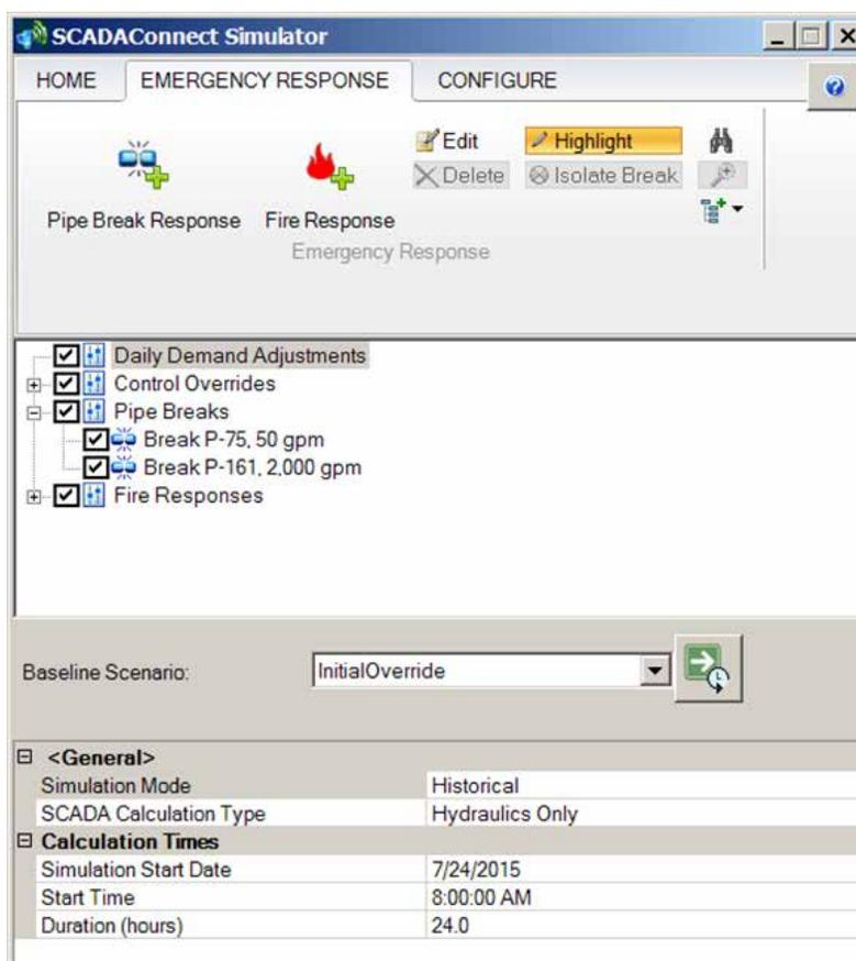
Figure 2: SCADAConnect Simulator provides an interface that operators can easily use to test various scenarios.
