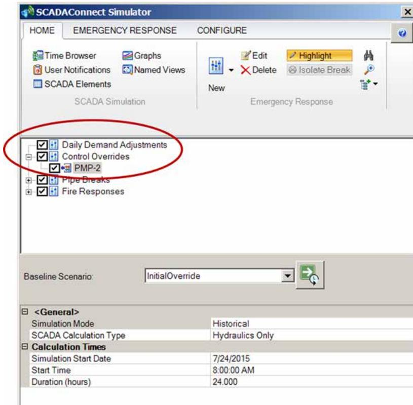
Figure 3: SCADAConnect enables you to easily adjust water demands and controls to predict and visualize network response.
